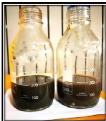
Figure 2. The dark brown colour of prepared biogenic Silver nanoparticles(AgNPs) after 48 hours of incubation.
